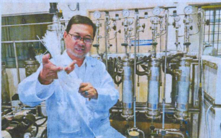
In use: Ahmad Fauzi with a test purification ensemble scaled down 10 times its actual size. The fibres work within steel chambers set with pressure gauges.
