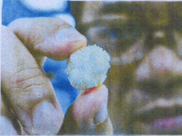
Straw-like: The fibres act like a sieve to allow only desirable materials to seep through its membrane. Output then travels along the inner hollow sections.
