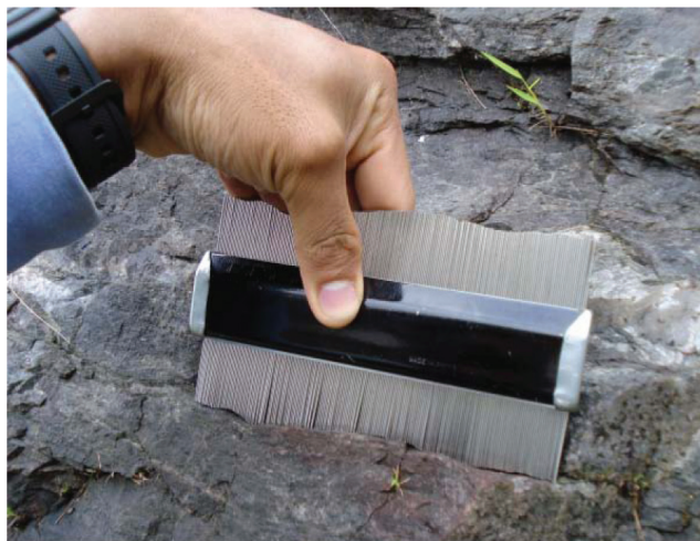
Figure 1. Profiler employed for the determination of JRC.
