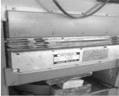
Figure 1. The hot compress machine used to form the boards.
