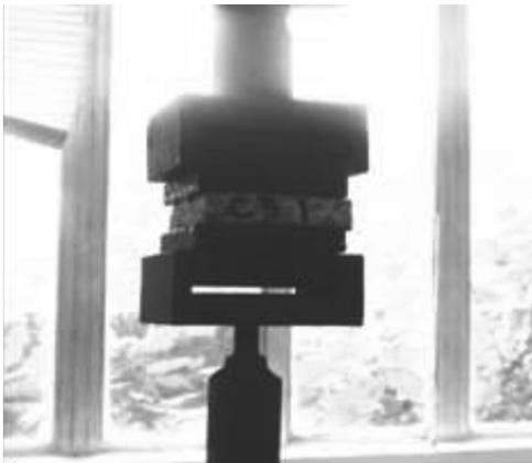
Figure 2. Test for internal bond strength.
