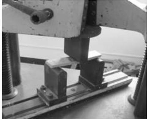
Figure 4. Test for screw holding capacity.
