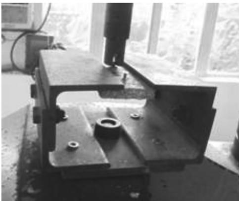
Figure 3. Test for modulus of rupture.
