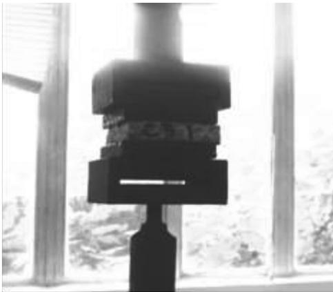
Figure 2. Test for internal bond strength.
